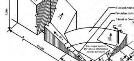
Note - Part 77.25 does not make provisions for precision approaches to utility runways. In these situations, use precision standards for other than utility runways to develop the primary, approach, and transition surfaces.
