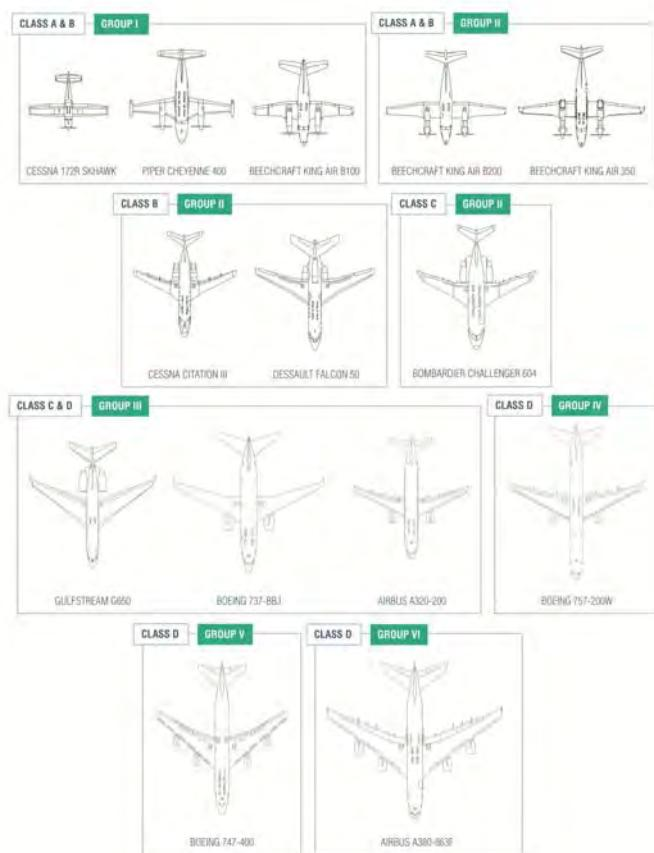
A Critical Aircraft is defined as the most demanding aircraft to regularly use the airport. Planners use Aircraft Design Group and Approach Categories that relate airport design criteria to the operational and physical characteristics of the airplanes that are intended to operate at an airport. The Critical Aircraft for Double Eagle II Airport falls within the C/D-II range.
