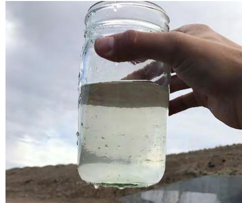
Stormwater grab sample taken from outfall being visually evaluated for presence of potential contaminants.
