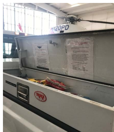
Mobile refueling truck well stocked with spill response materials and spill response plan.
