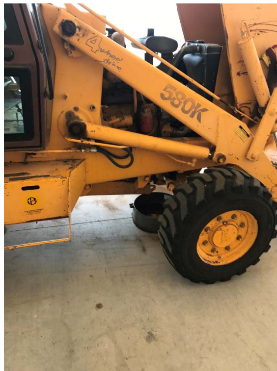
DEII Airfield Maintenance identified leaking equipment and moved it to the covered wash bay and placed a drip pan under the drip until the equipment could be serviced.
