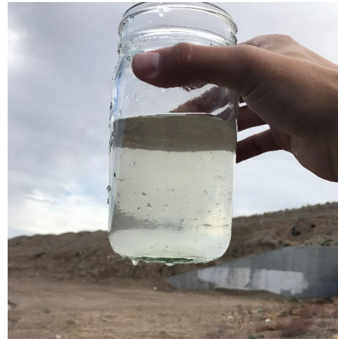
Stormwater grab sample taken from outfall being visually evaluated for presence of potential contaminants.
