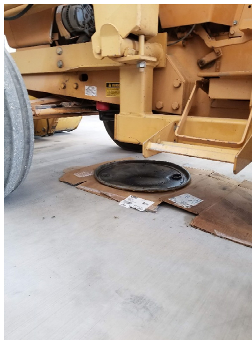
DEII Airfield Maintenance identified leaking equipment and moved it to the covered wash bay and utilized a drip pan until the equipment could be serviced.
